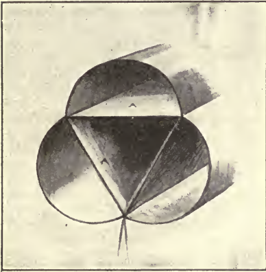
CROSS SECTION OF AN ASTRA-TORRÈS AIRSHIP, SHOWING MODE OF SUSPENSION
